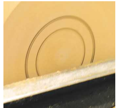
▲ Pic.6 For easy working Les is going to use a stepped spigot on the bowl. The smaller one is for the chuck which will be removed, and the larger one is the base of the bowl
